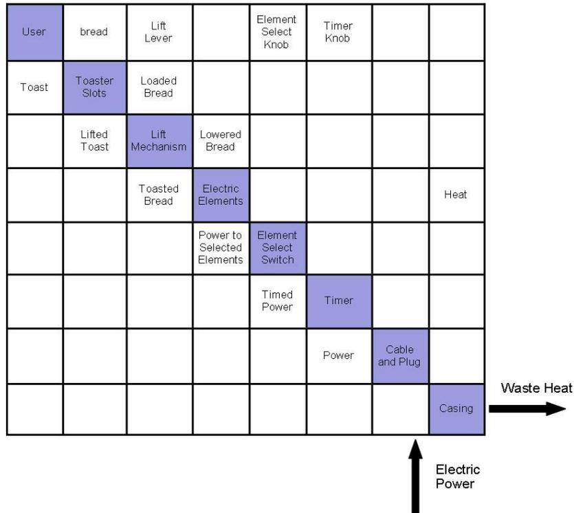
Figure 14: An N<sup>2</sup> Matrix for the Typical Domestic Toaster.
