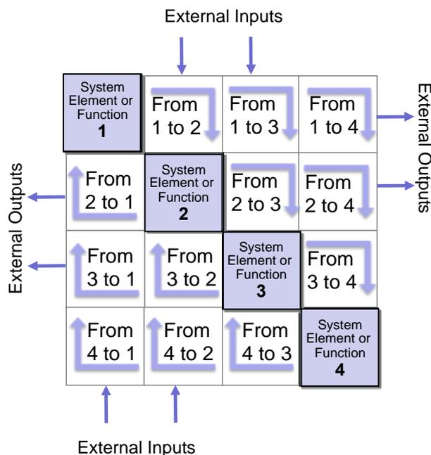
**Figure 3: The key features and rules of an N<sup>2</sup> matrix**
