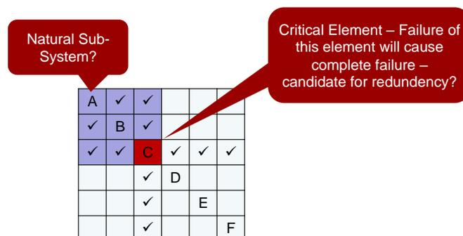
Figure 1: A Typical N<sup>2</sup> Matrix
