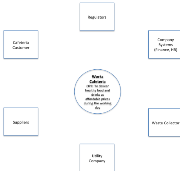
Figure 7: Identify all Possible Terminators first. Having identified the potential Terminators, each can be considered in turn to identify the potential flow interactions with the system of interest. The end result could look like Figure 8.
