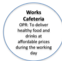
Figure 3: The starting point for drawing a Context Diagram: the System of Interest as a bubble with its Operational Requirements
