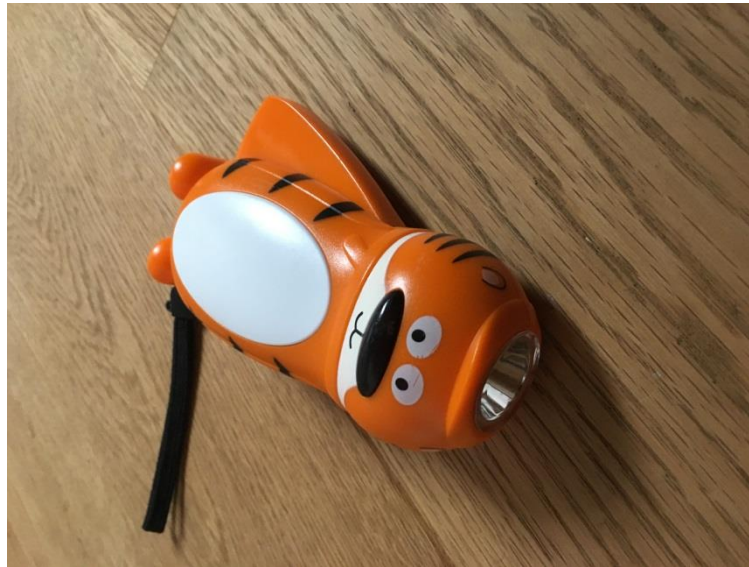
Figure 2: A tiger shaped hand generator LED torch
